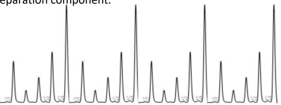
With injections being made at 1.4 min intervals (84 sec) and column switching every 7 min this platform can analyze ~40 samples per hour, i.e. ~1000 samples per day.
