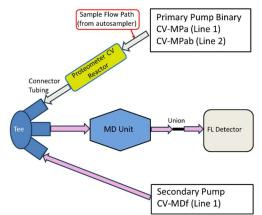
To avoid damage to the Proteometer-CV reactor, the flow rate of the primary pump must always be greater than or equal to the flow rate of the secondary pump
